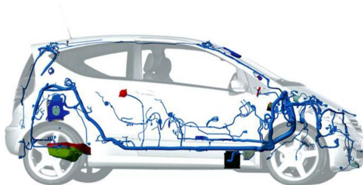
Figure 2. Automotive wiring system example
