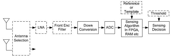
Fig. 4. Block diagram of the sensing module.
