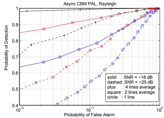
Fig. 8. Simulations: Probability of detection vs. probability of false alarm of PAL Sensing in Rayleigh fading channel based on CBM.
