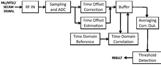
Fig. 5. Block diagram of PAL sensing.
