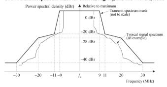
NOTE 1 - The outer heavy line is the spectrum mask for 802.11a, 11g, 11j, HiSWANa and the inner thin line is the envelope spectrum of OFDM signals with 52 subcarriers.
