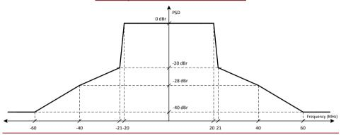
NOTE - The spectrum emission mask is defined relative to the maximum power density in a 1 MHz measurement bandwidth within the channel bandwidth. The relative power of any transmitter emission shall not exceed the levels indicated by the mask or –30 dBm/MHz whichever is the greatest.
