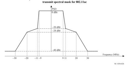
NOTE - For 802.11n, the maximum of -40 dBr and -53 dBm/MHz at 30 MHz frequency offset and above. For 802.11ac, the transmit spectrum shall not exceed the maximum of the transmit spectral mask and -53 dBm/MHz at any frequency offset.
