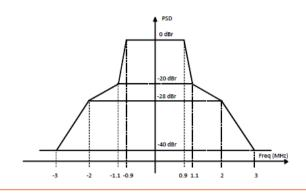
FIGURE 6c Transmit spectrum mask for 4 MHz 802.11ah channel
