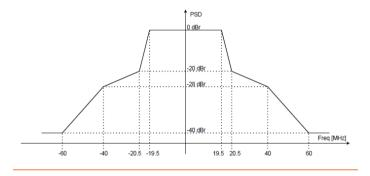
FIGURE 7c Transmit spectrum mask for 80 MHz 802.11ax channel
