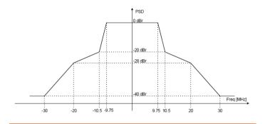
FIGURE 7b Transmit spectrum mask for 40 MHz 802.11ax channel
