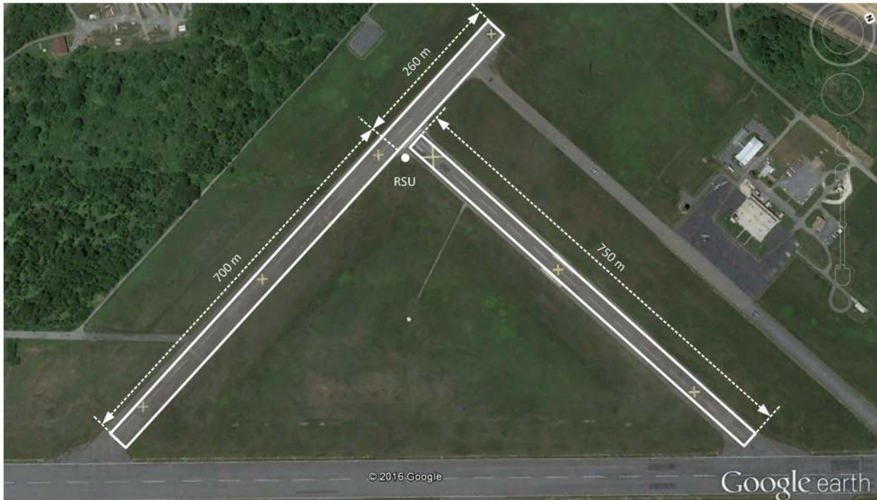
**Figure 5-1: Baseline Measurement Area for IEEE 802.11p and IEEE 802.11ac Radios**
