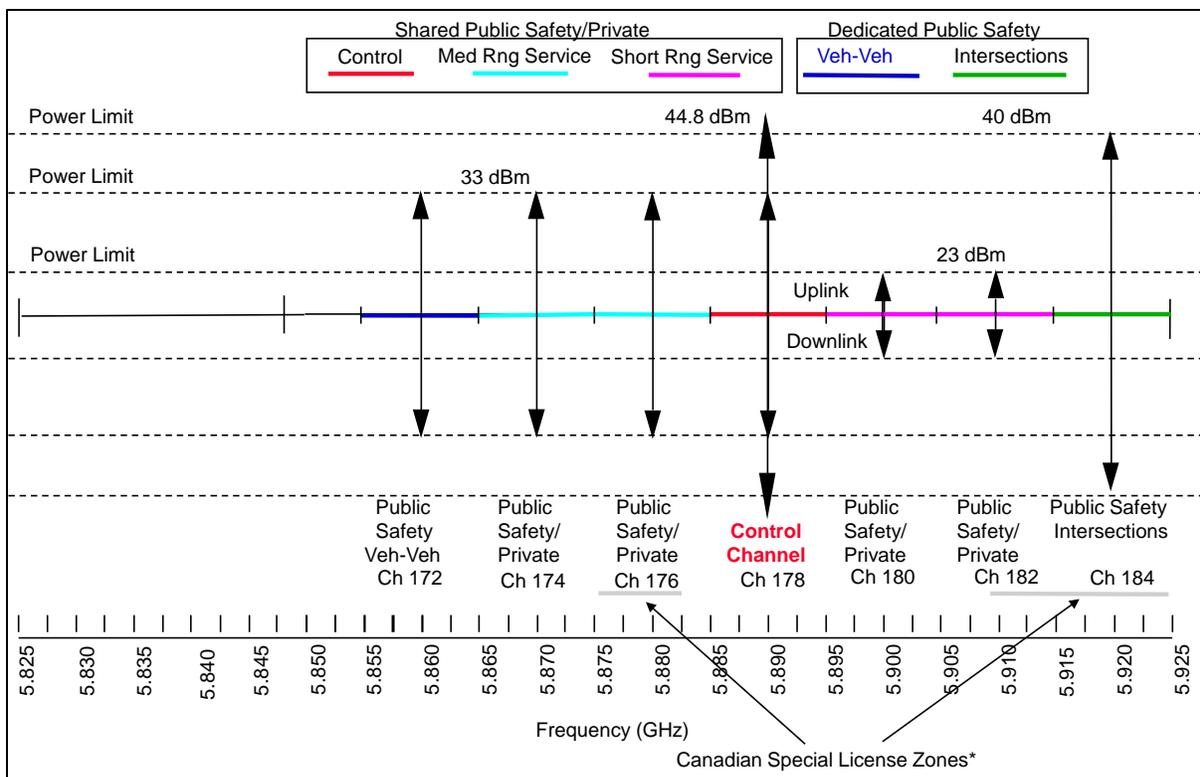
Figure 1-1: DSRC Channel Plan in the ITS Band<sup>13 14</sup>
