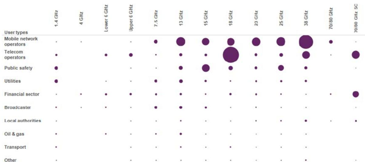
Figure 2: Indicative categorisation of Fixed Service spectrum<sup>20</sup> managed by Ofcom with usage shown by user types – the size of the circle is relative to the number of fixed wireless links licensed in the UK (based on fixed wireless link data of June 2016)
