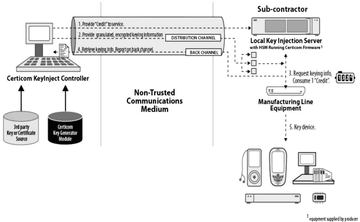
**Figure V-4 Secure device manufacturing in an untrusted environment**
