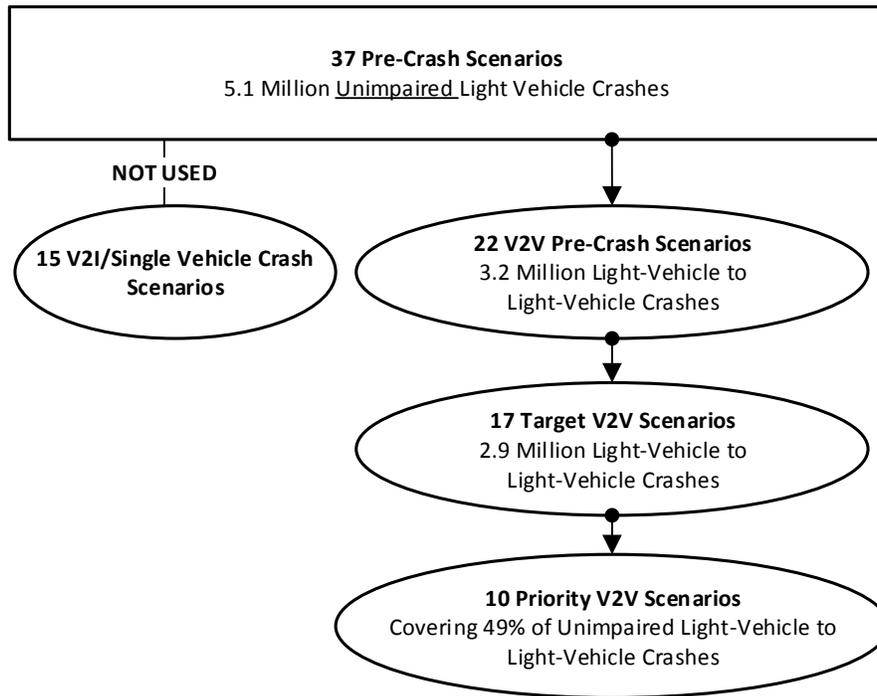
**Figure II-2 V2V Pre-Crash Scenario Breakdown<sup>16</sup>**
