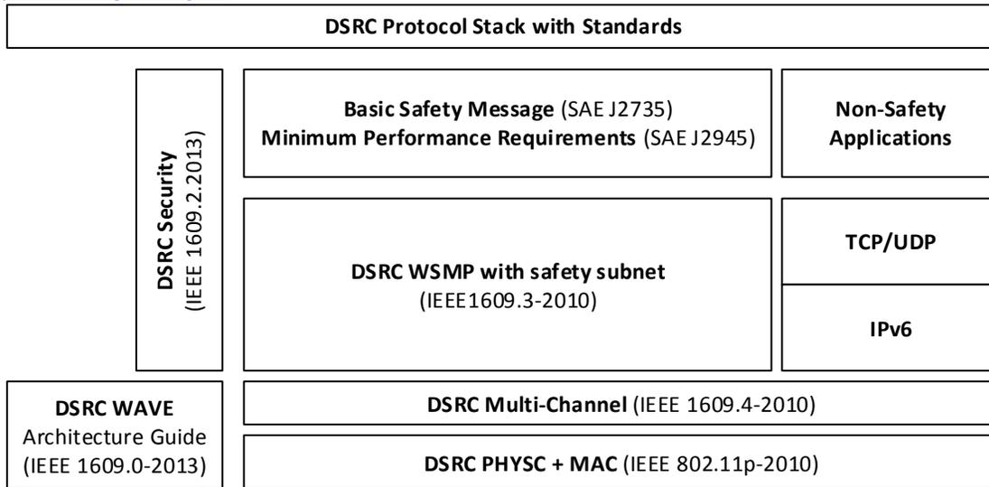
**Figure III-6 DSRC Protocol Stack**
