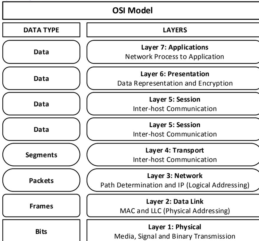
**Figure III-5 OSI Stack**
