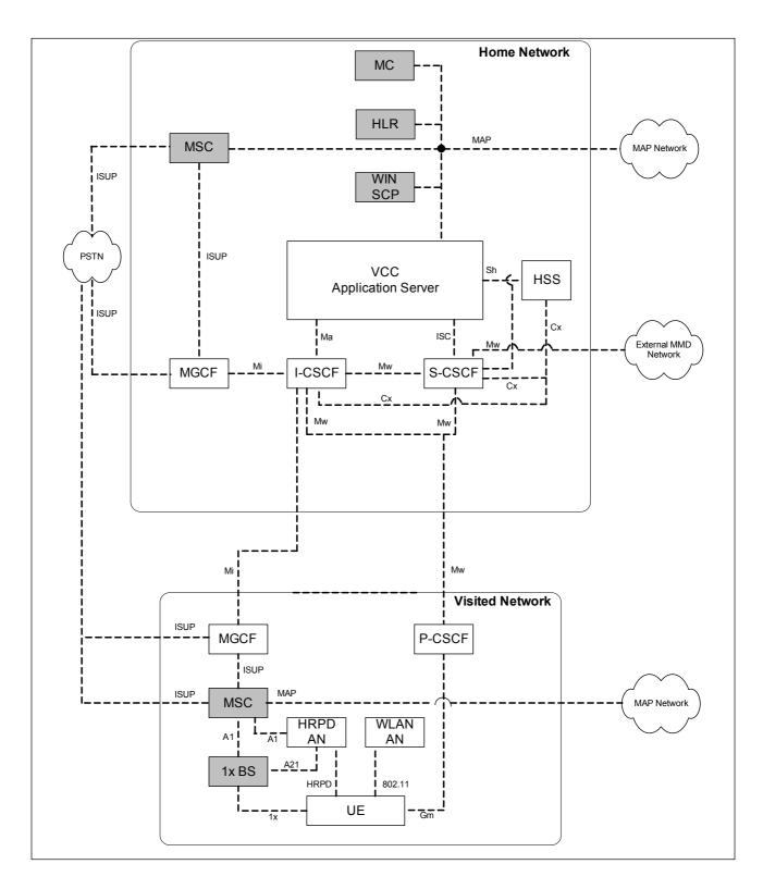
Voice Call Continuity introduces a new VCC Application Server (VCC AS) functional entity in the MMD network and relevant reference points for communication with the CS and IMS functional entities. The VCC AS makes use of existing CS and IMS functional entities and reference points.
