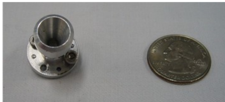
Conical horn antenna Beam-width 30 deg
