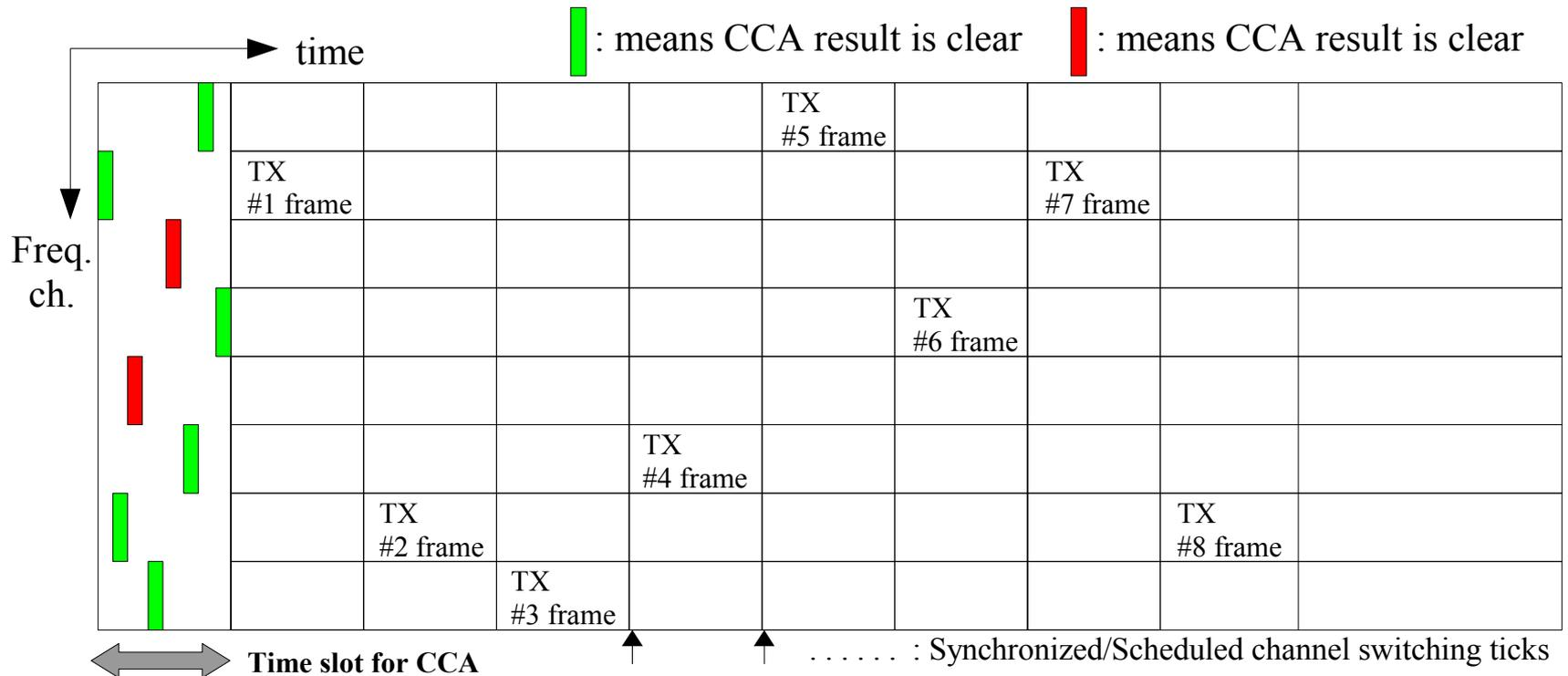
TX node must ensure at least a frame is following the previously scheduled channel and time slot unchanged to inform the new transmission channels and its order to send. Adaptive utilization of channels according to CCA is possible.
