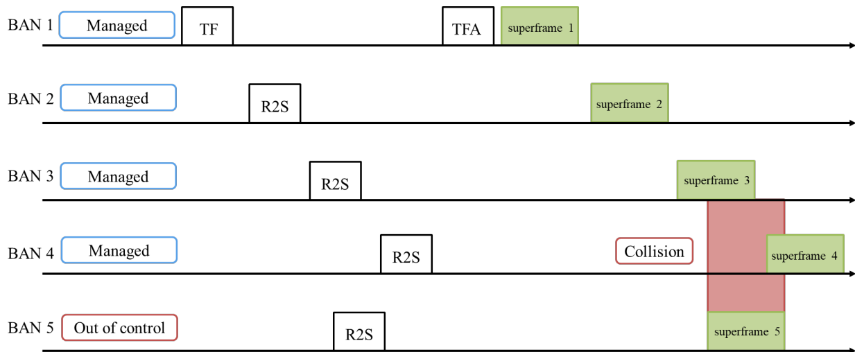
Figure 4— A Case of Four UWB BANs Synchronized but One Asynchronized out of Coexisting Five UWB BANs
