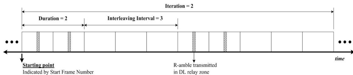
**Figure 6-7—R-amble transmission pattern as per the preplanned scheme instructed by MR-BS**
