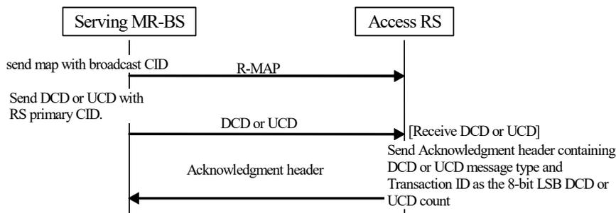
Figure 6-8—Relaying DCD/UCD procedure
