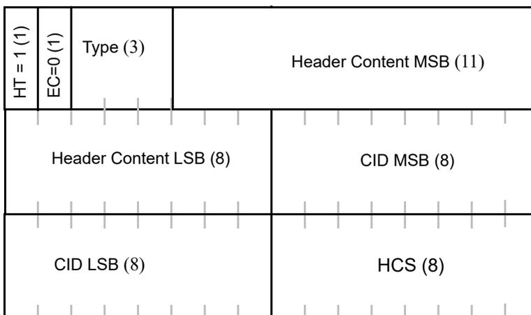
**Figure 6-5—MAC signaling header type I format**
