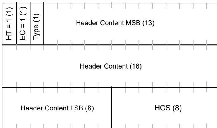
**Figure 6-6—MAC signaling header type II format**
