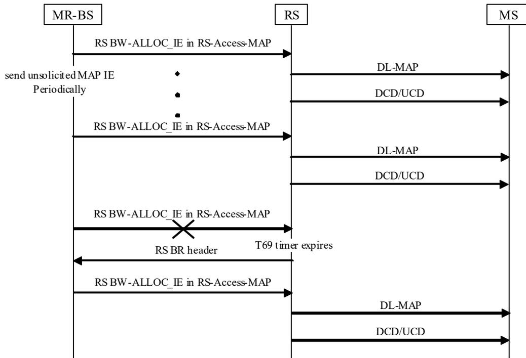
**Figure 6-9—DCD/UCD broadcasting procedure with an RS operating in centralized scheduling mode**
