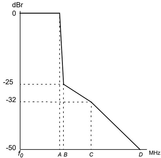
Figure 8-1—Tx spectral mask (see Table 8-2)
