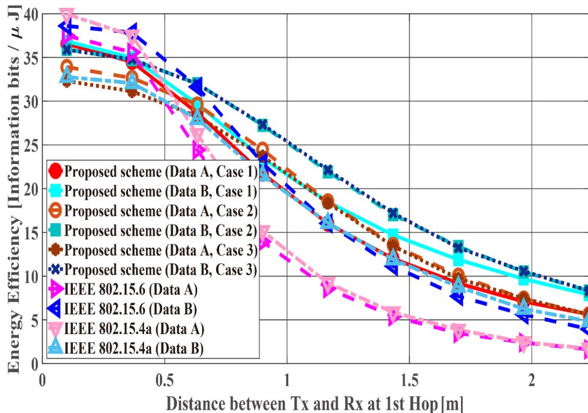
Energy efficiency with constant  $d_{2nd} = 40$  cm, the distance of the first hop  $d_{1st}$  is changed from 10 centimeters (cm) to 2.2 m
