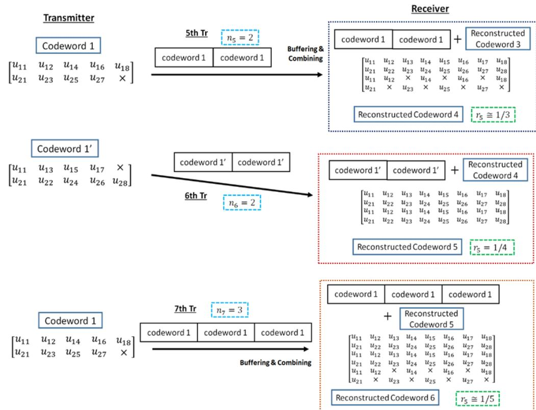
4. After that, codeword 1 and 1' are sent alternately  $n_i$  times and stored. Then, a receiver reconstructs and decodes low-rate decomposable codes by changing the number of data copies  $n_i$  in Weldon's ARQ protocol. At this time, a buffered old codeword is updated to a transmitted new codeword
