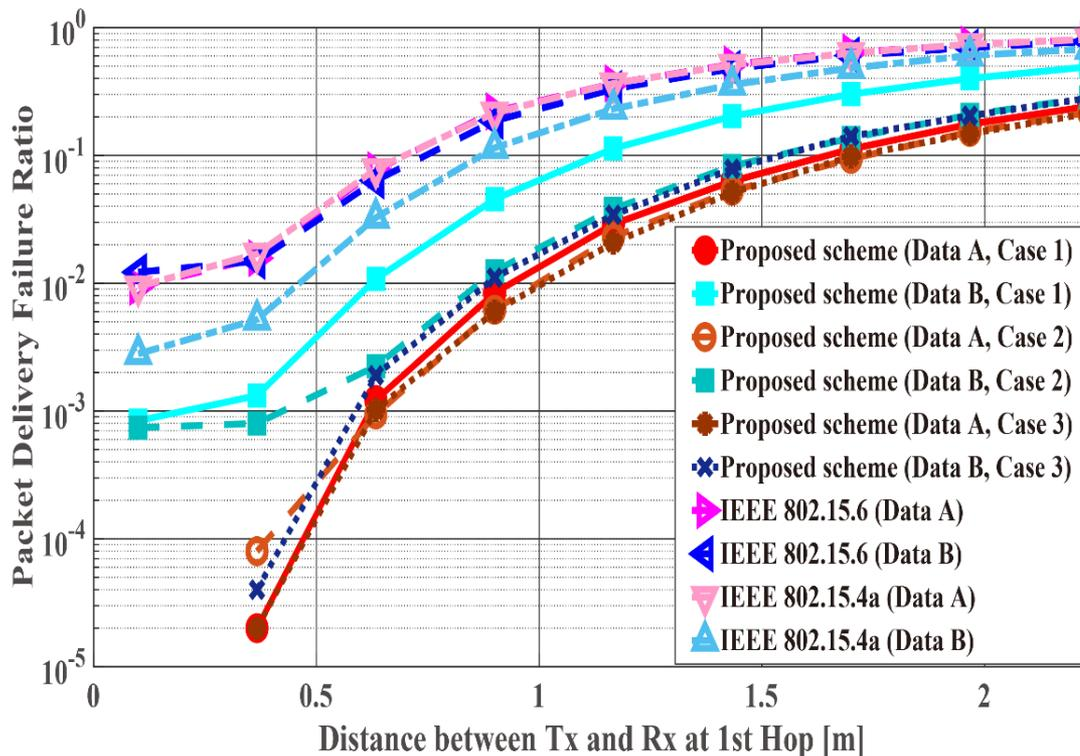
Packet delivery failure ratio with constant  $d_{2nd} = 40$  cm, the distance of the first hop  $d_{1st}$  is changed from 10 centimeters (cm) to 2.2 m
