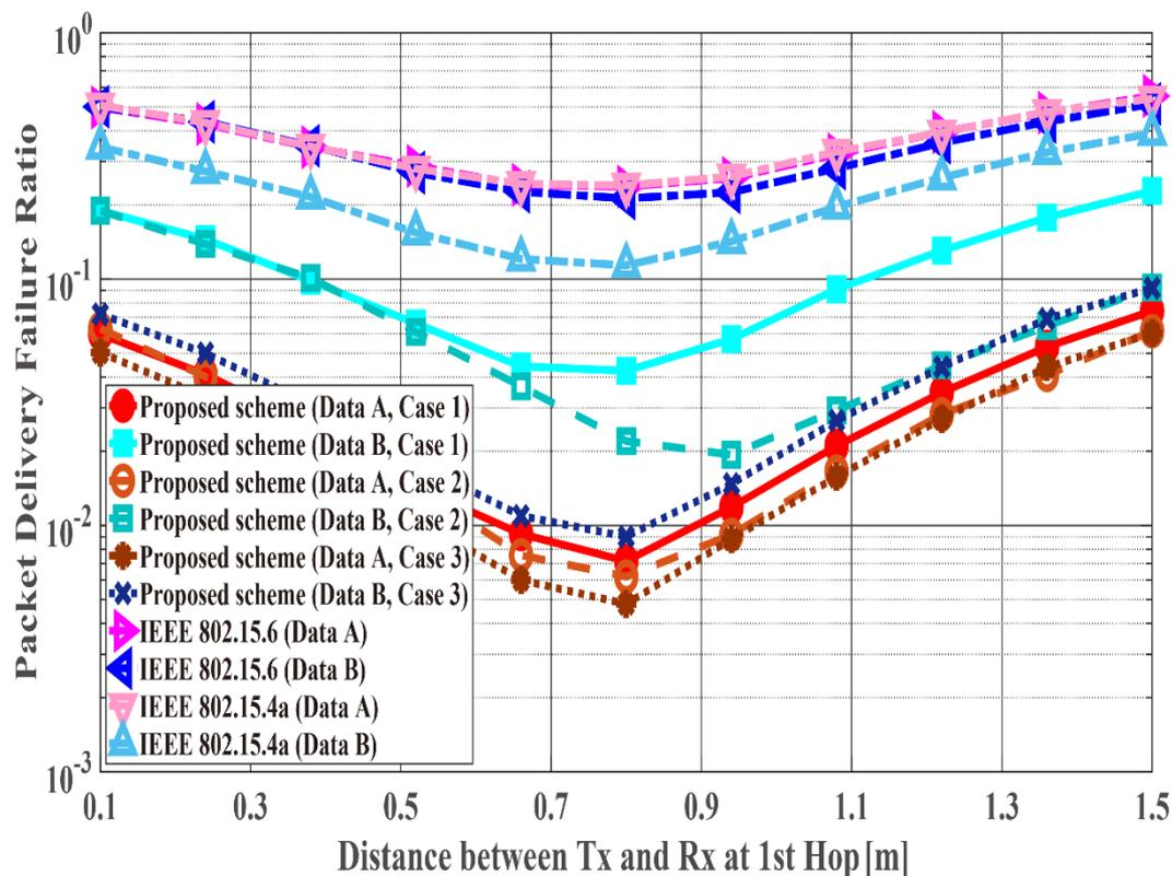
Packet delivery failure ratio with constant  $d_{2hops} = d_{1st} + d_{2nd} = 1.5$  m varying the  $d_{1st}$  and  $d_{2nd}$  values. For  $d_{1st} = 1.5$  m, data are transmitted using only a single hop.
