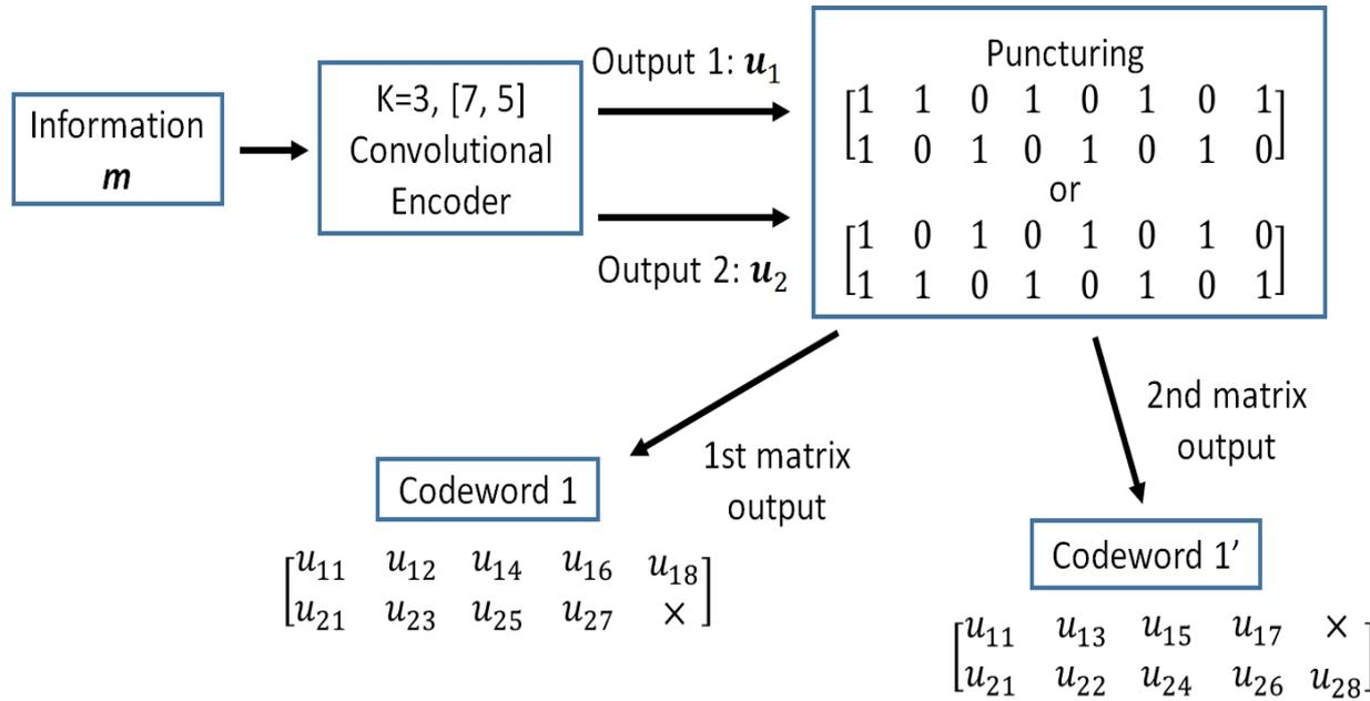
1. Firstly, the information bit sequence  $m$  is encoded via the punctured convolutional code, and codeword 1 is transmitted
