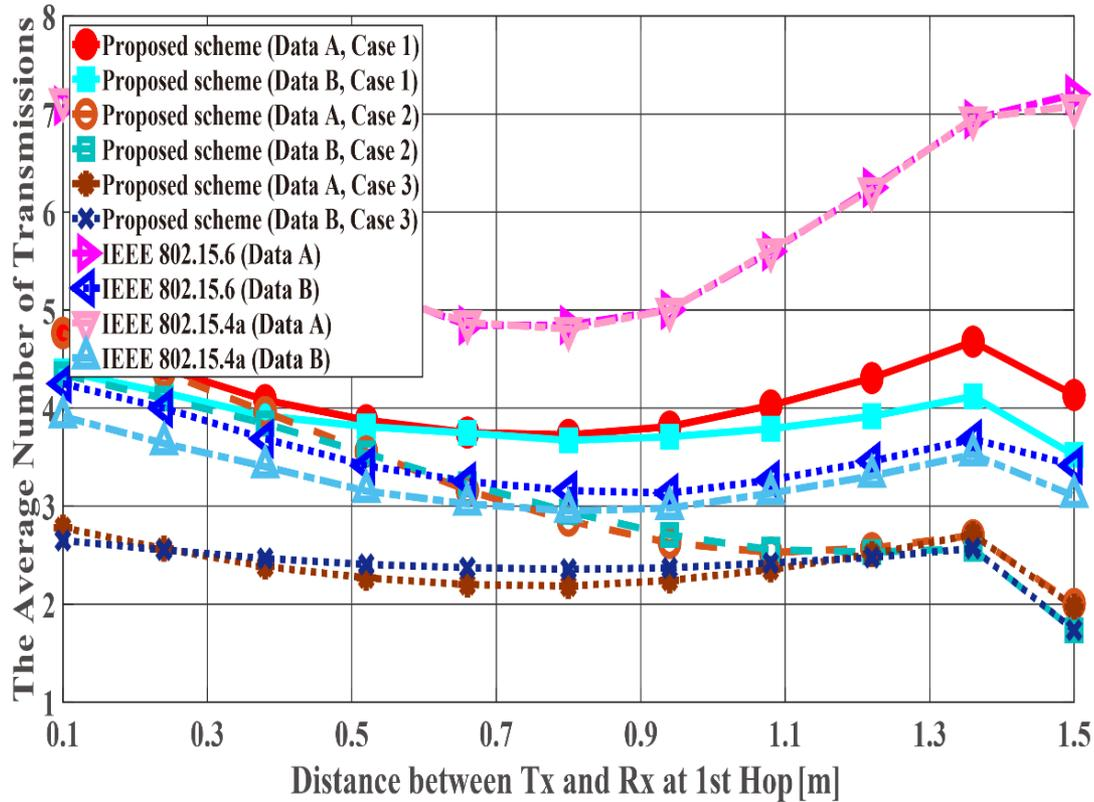
Average number of transmissions with constant  $d_{2hops} = d_{1st} + d_{2nd} = 1.5$  m varying the  $d_{1st}$  and  $d_{2nd}$  values. For  $d_{1st} = 1.5$  m, data are transmitted using only a single hop.
