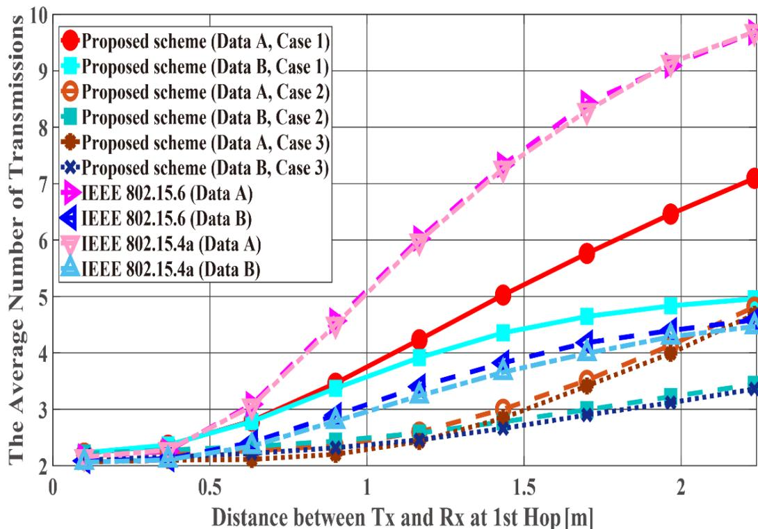
Average number of transmissions with constant  $d_{2nd} = 40$  cm, the distance of the first hop  $d_{1st}$  is changed from 10 centimeters (cm) to 2.2 m
