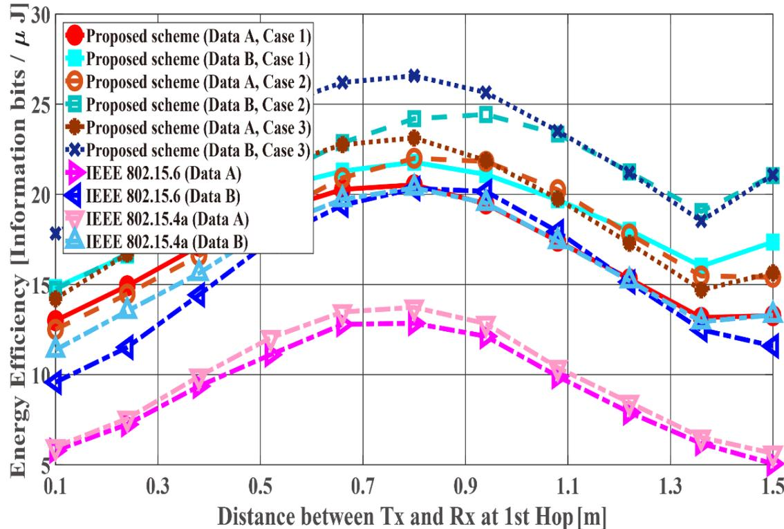
Energy efficiency with constant  $d_{2hops} = d_{1st} + d_{2nd} = 1.5$  m varying the  $d_{1st}$  and  $d_{2nd}$  values. For  $d_{1st} = 1.5$  m, data are transmitted using only a single hop.
