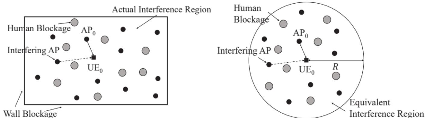
(d) The shape of an actual interference region. (e) Approximate interference region: an equivalent circle.
