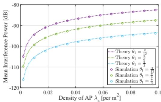
(a) Mean interference power versus the density of AP, varying  $\theta_1$ .
