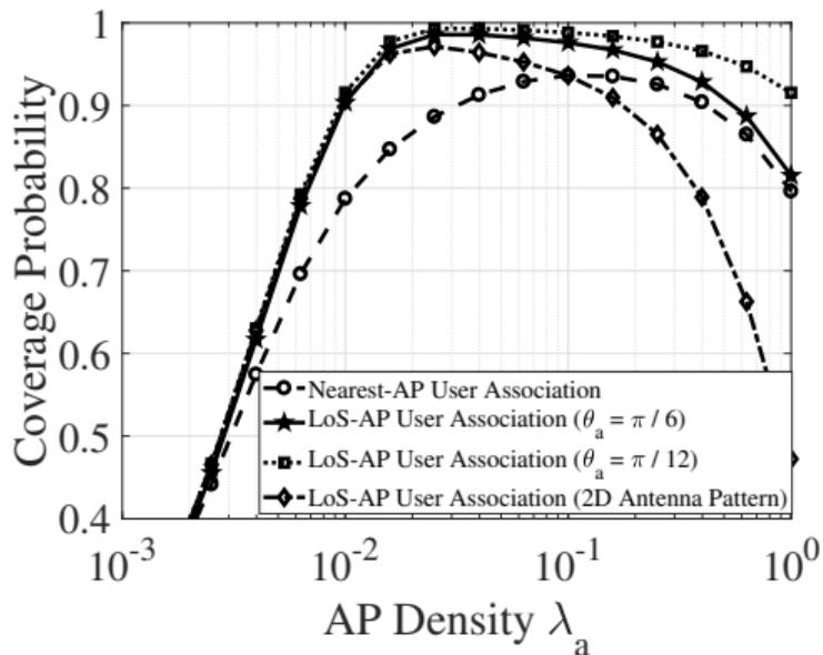
Figure: Coverage probability versus the AP density for SINR threshold  $T = 5$  dB.
