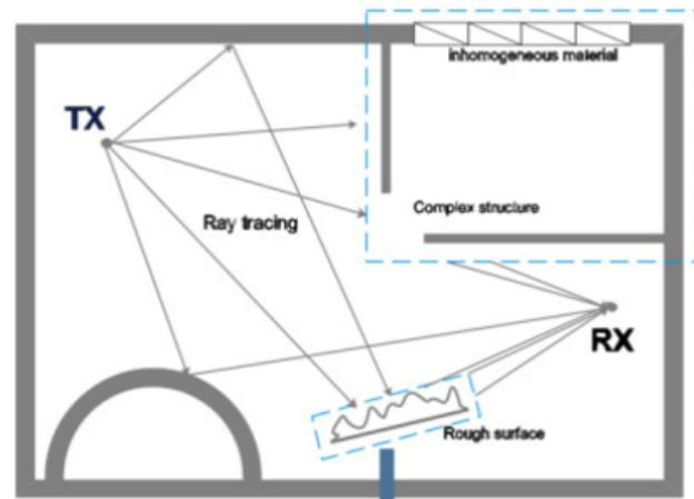
We use ray tracing to simulate the channels in the channel measurement campaign.
