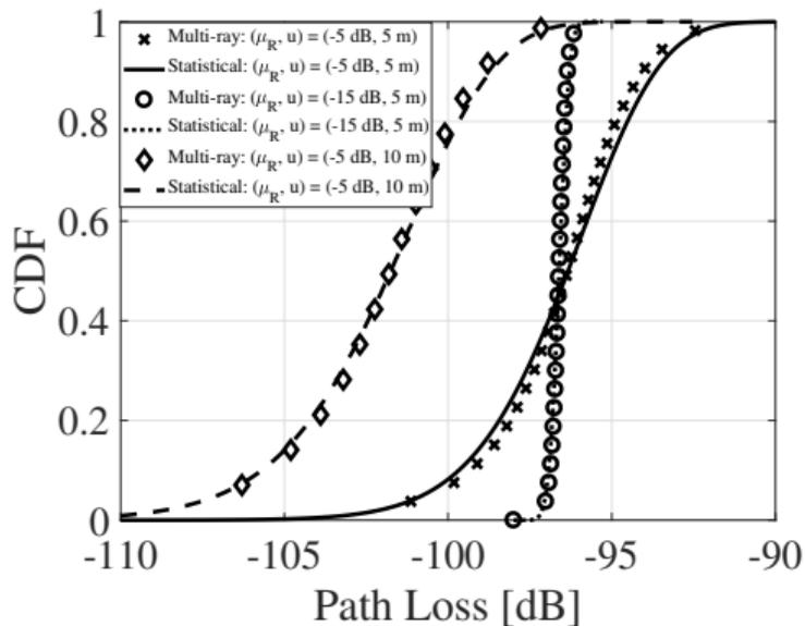
Figure: Comparison between the multi-ray model and the equivalent statistical model: LoS case.
