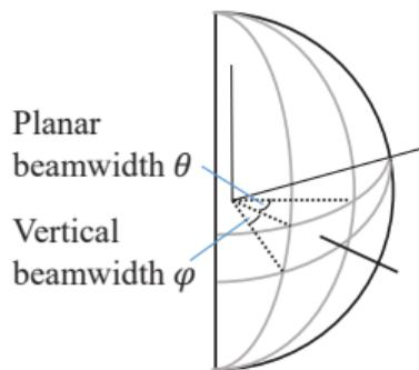
Figure: A pyramidal shape model of the antenna beam.
