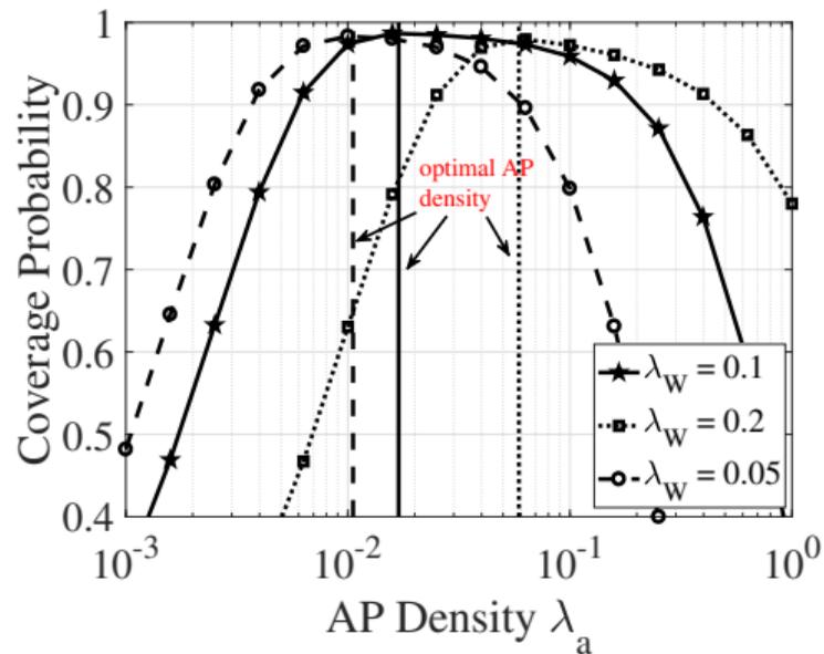
Figure: The optimal AP density versus the wall density.
