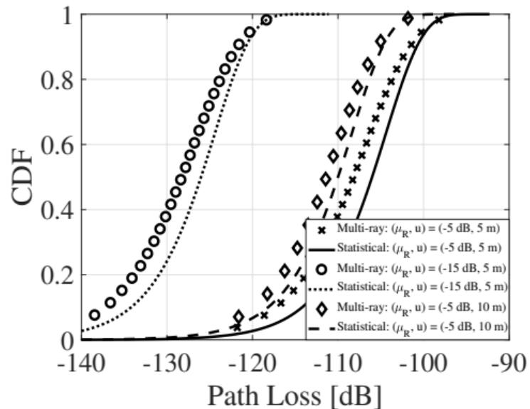
Figure: Comparison between the multi-ray model and the equivalent statistical model: NLoS case.
