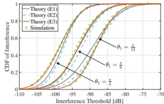
(c) Interference CDF with three ways of parameter fitting, varying  $\theta_1$ ,  $\lambda_a = 0.06$  per  $m^2$ .
