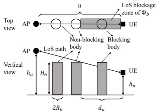
**Figure:** Top and vertical views of the human-blocking scenario for an AP-UE link.
