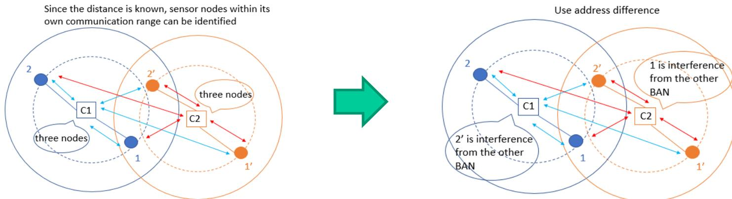
Fig4. how to identify overlap situations
