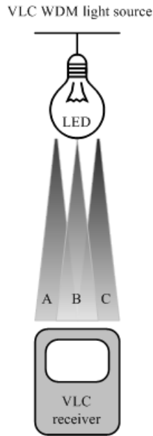
Figure F.3—A VLC application using WDM technology
