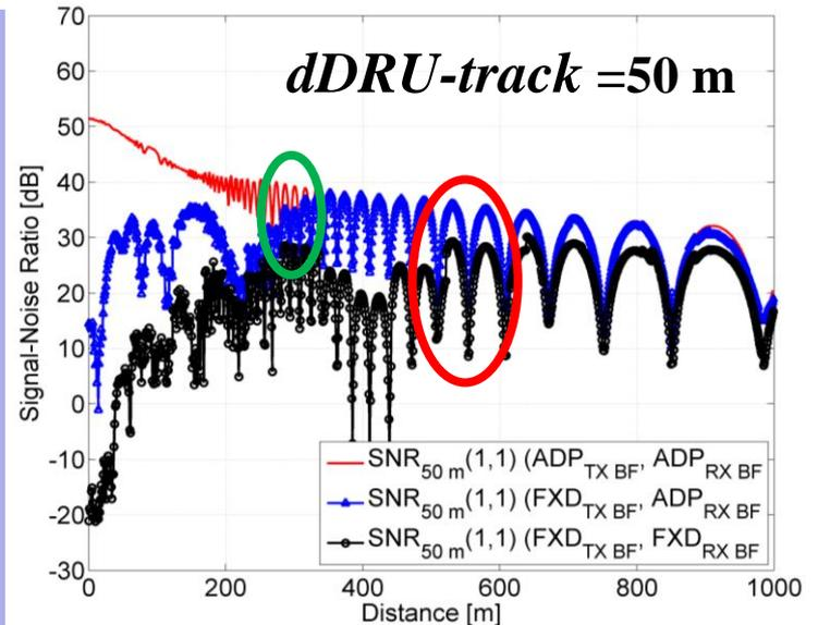
In the typical urban scenario, the adaptive BF on both sides provides the best channel:
