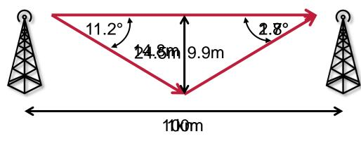
d=9.9 m @100 m distance for 10° HPBW d=24.5 m @1 km distance for 2.5° HPBW d=14.8 m @1 km distance for 1.5° HPBW
