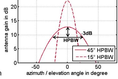
Assuming a Gaussian antenna pattern in elevation and azimuth:
