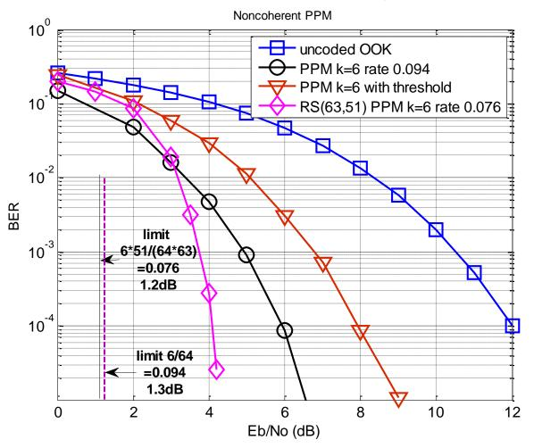
RS coded PPM has better performance than uncoded PPM in AWGN channel. RS(63,51) with PPM k=6 has a performance close to the Shannon limit
