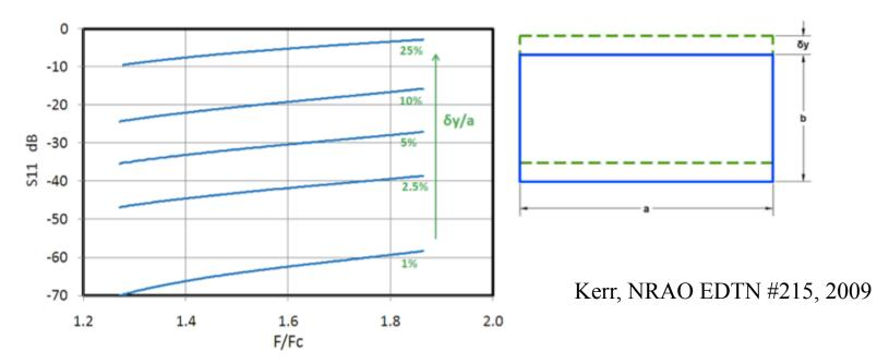
Fig. 4. Effect of flange misalignment of rectangular waveguides with 2:1 nominal aspect ratio. Only misalignment in the b direction is considered because misalignment in other directions has a smaller effect.
