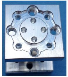
Experimental Waveguide Interface (500-750 GHz)
