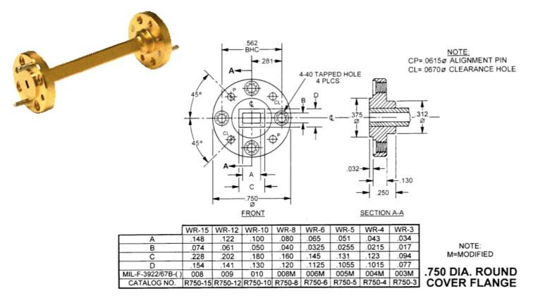
Fig. 1 The MIL Spec 0.75" round flange (UG-387 type) (from the Custom Microwave catalog). Dimensions in inches.
