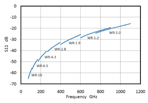
Fig. 4. Reflection at a waveguide joint with a 0.001" (25  $\mu$ m) misalignment in the *b* direction, for several waveguide bands (simulated [7]).
