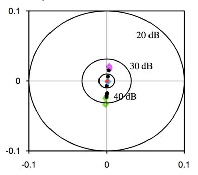
(c). Complex S11 on a Smith Chart at 625 GHz. The pink, green, and light blue empty diamonds are measurements with the flanges pushed in the H- and E-planes, and in rotation, respectively, while tightening the screws. The ten black dots represent the disconnection/re-connection data. And the red dot is the initial measurement before disconnection of the load.
