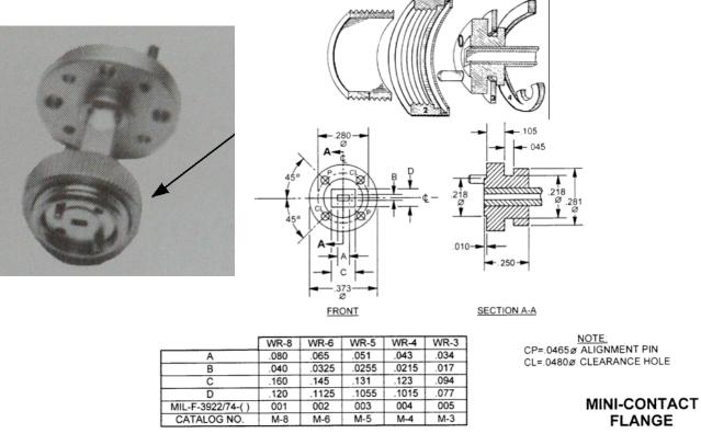
Fig.2. The MIL Spec mini-contact flange (TRG-714 type) (from the Custom Microwave catalog). Dimensions in inches.
