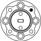
Ring-centered interface -- using UG-387 outer pins
