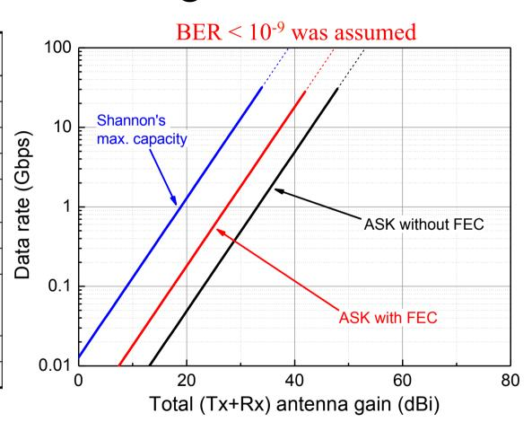
For 20 Gbps, Tx/Rx antennas together should provide more than 46-dBi gain
