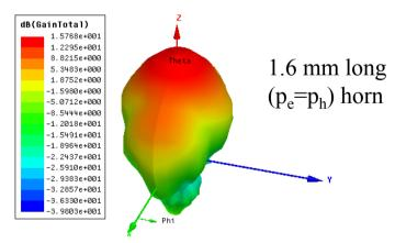
12~16 dBi gain antenna would be available in a couple of millimeter thick dimension.
