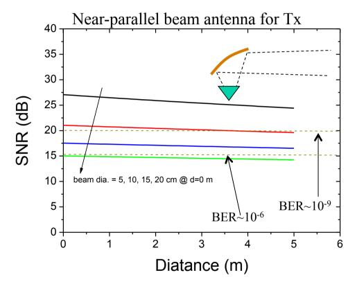
Near-parallel beam antenna will help to make the link more tolerant to the beam alignment even with no automatic beam streering.
