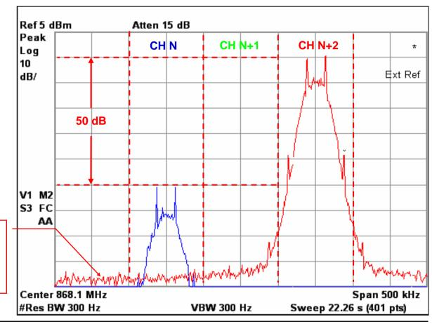
Phase noise of interferer (R&S SMIQ) bleeds into wanted channel
