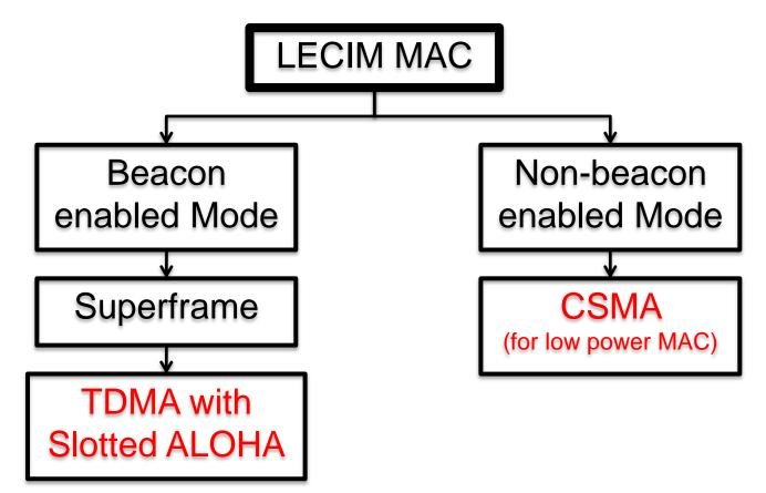
• CCA - even though not very effective – comes with little additional cost and it is used in non-beacon enabled mode for generality.
