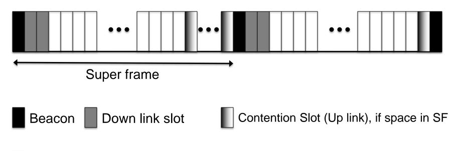
TDMA slot (Up link), assigned based on DEVID & Beacon sequence No.
