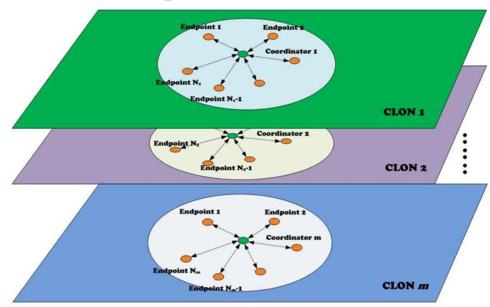
CLONs can use different frequency bands (channels) with different center frequencies;
