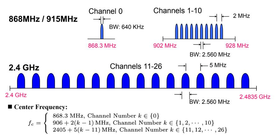
■ Like the IEEE STD 802.15.4 – 2006, if we use a roll-off coefficient  $\beta = 1$ , the RF bandwidth will be correspondingly 640 KHz and 2.560 MHz, respectively.
