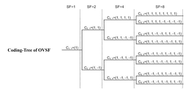
Note that for better system performance in interference mitigation, robustness in multipath fading, and synchronization, Gold or m sequence based scrambling can be jointly used with OVSF.
