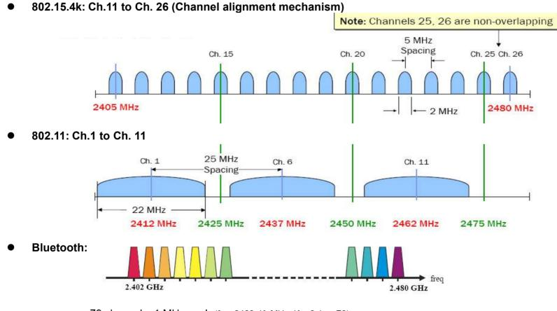
79 channels, 1 MHz each (fc = 2402+K MHz; K = 0,1,....78) Frequency hopping (1600 hops/s)
