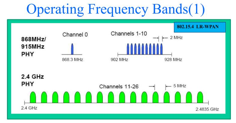
■ Totally, there are **3** applicable frequency bands and **27** channels with different bandwidth
