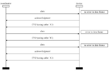
Figure 36—CVD frame usage for acknowledgment indication
