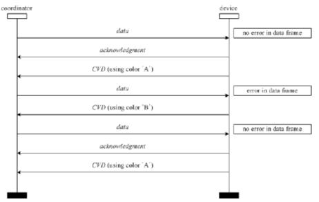
Figure 36—CVD frame usage for acknowledgment indication
