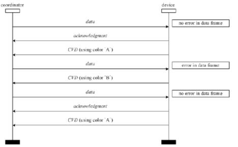
Figure 36—CVD frame usage for acknowledgment indication
