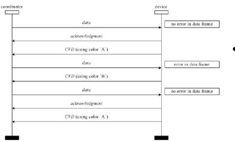
Figure 36—CVD frame usage for acknowledgment indication
