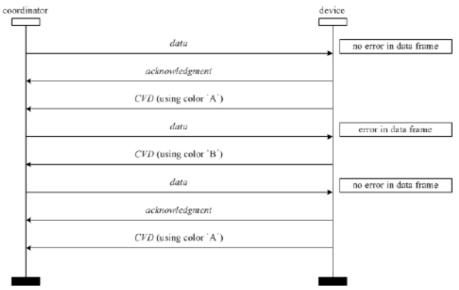
Figure 36-CVD frame usage for acknowledgment indication
