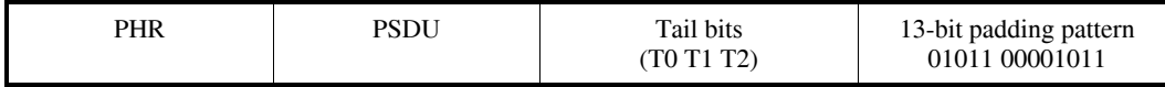
Figure 65t—An example of extension with padding bits prior to encoding, when (L_{PHR} + L_{PSDU})/8 is even
