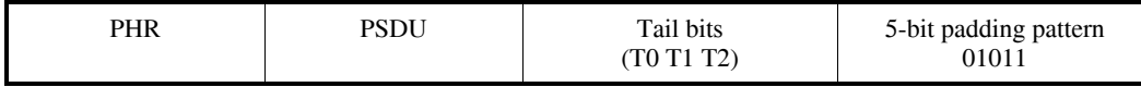
Figure 65s—An example of extension with padding bits prior to encoding, when (L_{PHR} + L_{PSDU})/8 is odd
