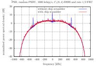
▶ relevant for operation at max. power in 902-928 MHz band (FCC §15.247: spectral density limit of 8 dBm/3 kHz).
