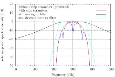
AWGN 868.3 MHz, 100 kchip/s,  $(8,1)_{0/1}$ -DSSS and rate 1/2 FEC, 64 octets
