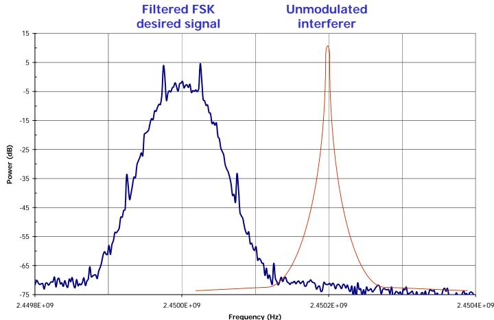
Adjacent channel rejection test as specified by P802.15.4g/D2
