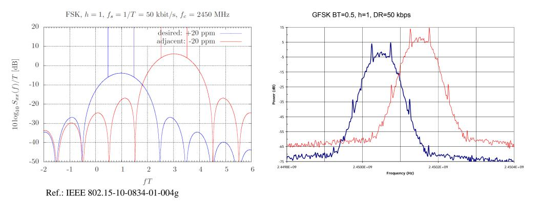
• GFSK ('filtered FSK') with strong attenuation of the sidelobes provides a significant advantage also in situations with large frequency tolerances.
