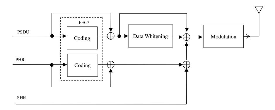
\* When FEC is enabled, PHR and PSDU shall be coded as a single block of data, as described in < Insert correct subclause number>
