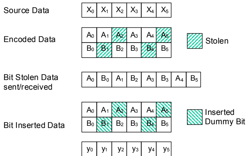
Figure 65h—Puncturing for rate 3/4
