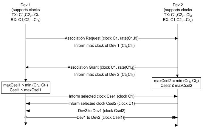
There is a data rate table <u>rate{Ci,j}</u> associated with each clock rate Ci where j is the data rate index associated with clock rate Ci
