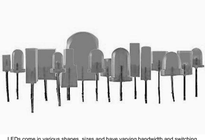
LEDs come in various shapes, sizes and have varying bandwidth and switching frequencies from 100's of KHz to 100's of MHz
