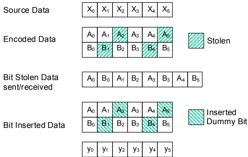
46 Figure 65t—Puncturing for rate 3/4
