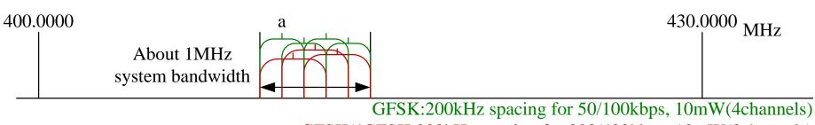
GFSK/4GFSK:200kHz spacing for 200/400kbps, 10mW(3channels)
