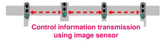
The Traffic Signal Sub Project started studies about the use of the visible light communication to control information transmission between traffic signals using image sensor receivers
