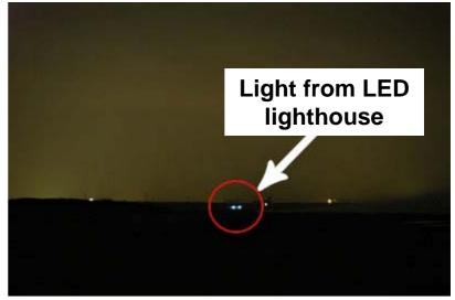
VLCC succeeded in the world record of long-distance telecom experiment by the visible light communication using image sensor communications technology
