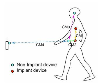
Fig. 1: Possible communication links for Body Area Networking
