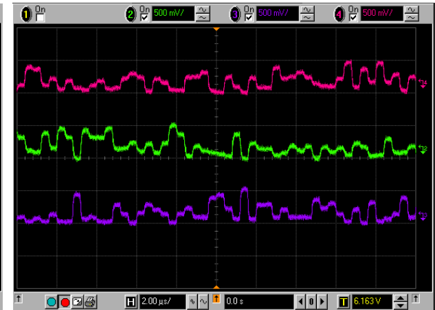
Demodulated Signal Symbol for CMC with symbol points (datadem)
