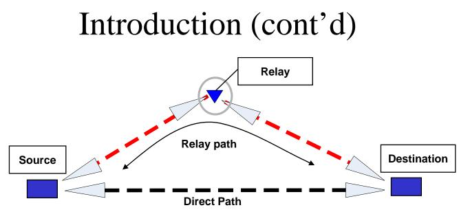
[Configuration of a pair of devices and a relay]
