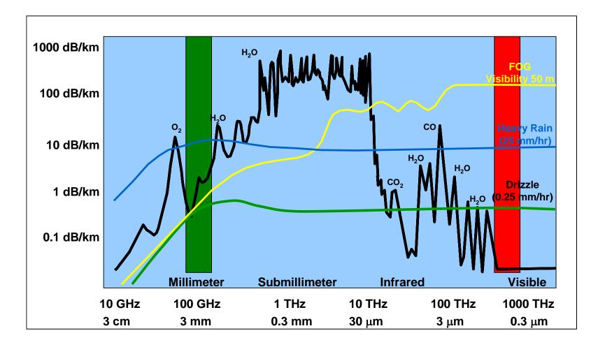
Millimeter-wave frequencies offer good transmission through fog, clouds and rain
