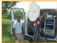
In August 2007, Battelle completed a field test to demonstrate 10 GB/s data transmission at 94 GHz.
