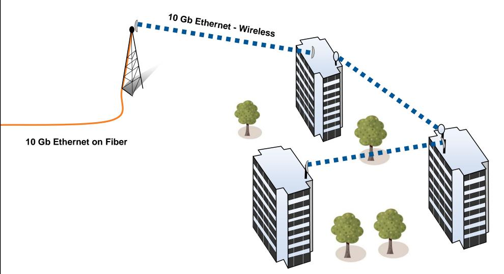
Battelle has developed a method to transmit 10 Gb/s over a wireless link. The application allows the wireless transport of 10 Gb Ethernet at distances to 2-5 km.
