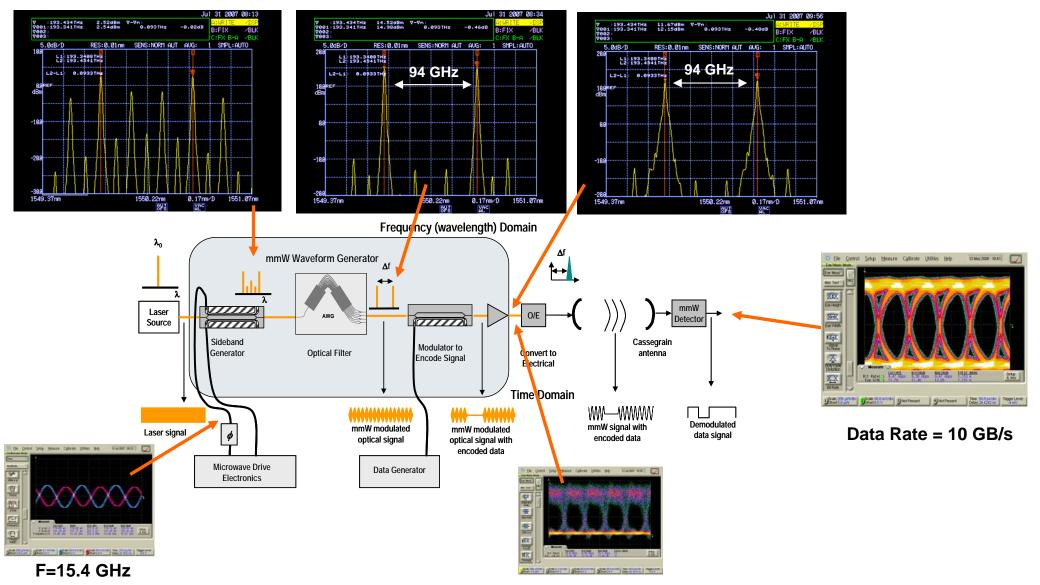
Battelle's IR&D Program is focused on the use of photonic components for the analog and digital modulation of millimeter-waves.
