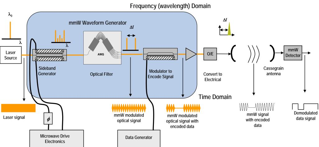
This block diagram outlines a wireless communication system capable of transmitting data in excess of 10 GB/s that uses an over-driven modulator to generate multiple sidebands. Various modulators, including lithium niobate and electrooptic polymer modulators, have been used to generate sidebands and encode data.
