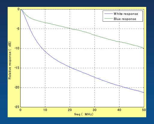
**Measured LED small-signal bandwidth**
