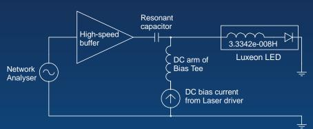
A single resonant driving circuit
