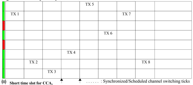
Even in this uncertain future scenario, TX node is supposed to include at least TX side information of channel usage by which RX node is able to be ensured if intended frame transmission have succeeded or failed. Simultaneous reception of multichannel at RX node would greatly improve the reliability of AFA.
