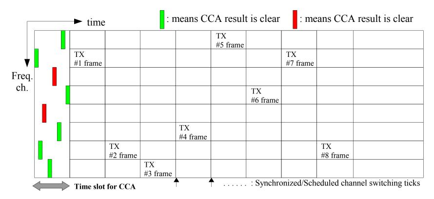
TX node must ensure at least a frame is following the previously scheduled channel and time slot unchanged to inform the new transmission channels and its order to send. Adaptive utilization of channels according to CCA is possible.
