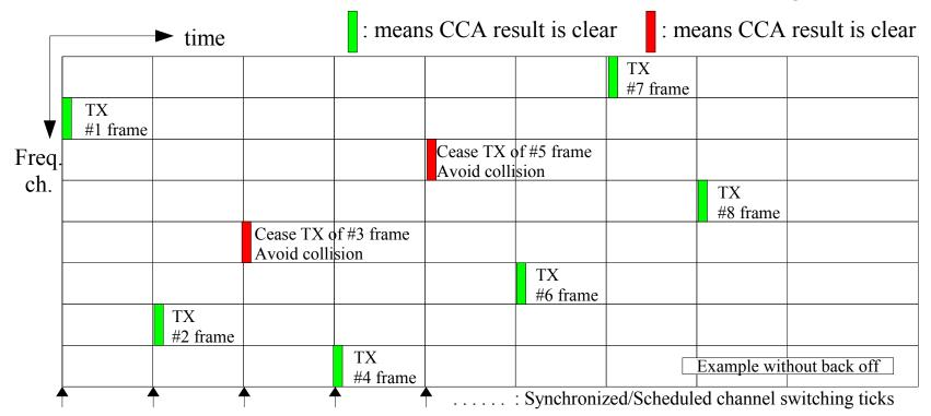
Then TX node must follow the pre-defined TX channel order to send. In this case, AFA means just CA, i.e., collision avoidance.
