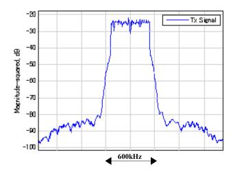
[ Simulated PSD example of signal ]
