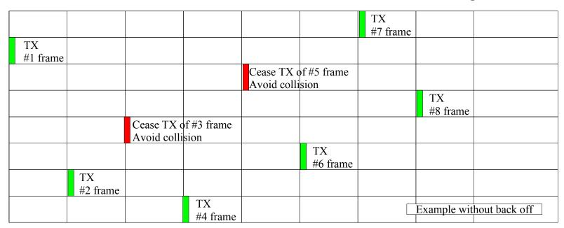
Then TX node must follow the pre-defined TX channel order to send. In this case, AFA means just CA, i.e., collision avoidance.
