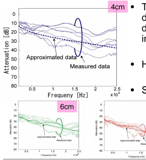
The gradient of approximated data gets sharper as the distance between antennas is increased
