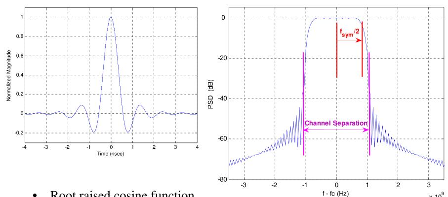
Root raised cosine function with roll-off factor 0.25
