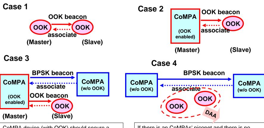
CoMPA device (with OOK) should secure a time slot as a PNC in the CoMPAs' superframe at first and should send a beacon to OOK with that time slot information to assure coexistence. If there is an CoMPAs' piconet and there is no OOK enabled CoMPA device, OOKs should avoid conflict according to the DAA manner
