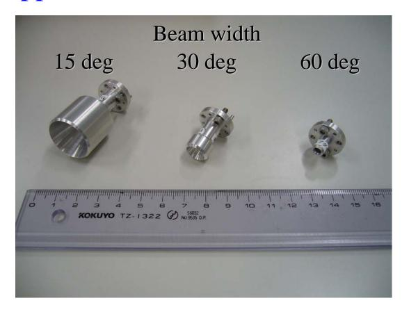
These antennas were used in channel measurement
