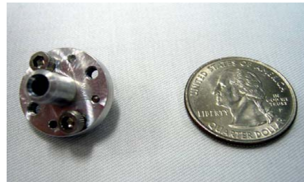
Conical horn antenna Beam-width 60 deg
