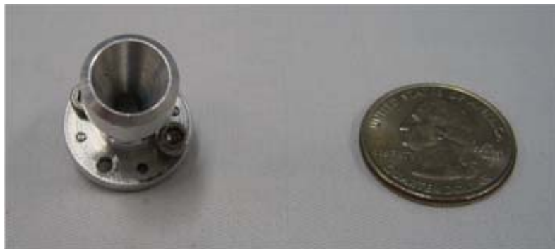
Conical horn antenna Beam-width 30 deg
