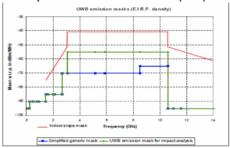
Fig. 2 Switzerland Proposed Mask to ITU-R TG1/8
