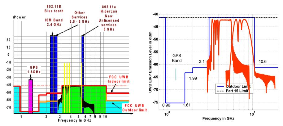
Ref. Modified pulse shapes based on SSA for interference mitigation and systems coexistence (update), Doc: IEEE 802.15-03-0457-00-003a
