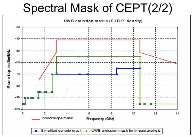
Fig. 2 Switzerland Proposed Mask to ITU-R TG1/8
